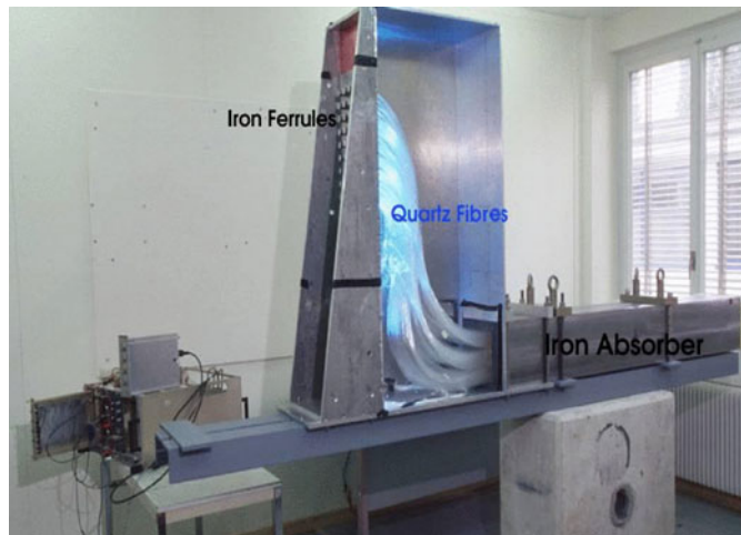
Figure 3. PPP-I before it was moved to H4 beam line at CERN. The 1.65 m long iron absorber is seen on the right. The quartz fibres are also seen coming off the absorber and bundling at the iron ferrules.
