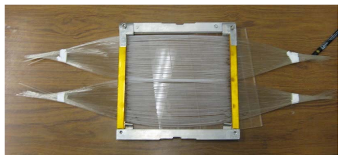
Fig. 12. The ribbon built with radiation hard WLS fiber prototype.
