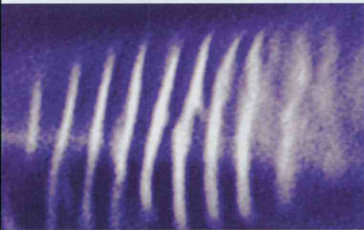
Figure 3. A dust acoustic wave propagating in a plasma shows up in a video image of light scattered by dust clouds in the plasma. The bright bands are compression wavefronts. Ordinary plasma waves in dustless plasmas cannot be visually imaged in this way. The wave is essentially a sound wave in the charged dust component of the plasma. Because the wave propagation involves the dynamics of the heavy dust particles with small charge-to-mass ratios, it's very slow (a few centimeters per second) and its frequency is only on the order of a hertz. By contrast, ion-acoustic waves in the plasma travel at kilometers per second. (Adapted from A. Barkan et al., Phys. Plasmas 2 , 3563 (1995).)
