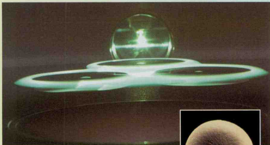
Figure 2. Rings of dust particles encircling silicon wafers in a plasma processing device. In an accidental 1989 discovery, laser light was shone into a plasma used to etch Si wafers so that the expected weak optical fluorescence would monitor concentrations of reactive gas. Instead, the fluorescence was overwhelmed by scattering of the incident light off unanticipated clouds of micron-sized particles electrically suspended in the plasma above the wafers. 4 Although great pains had been taken to minimize dust contamination of the clean room, it was discovered that the particles actually formed and grew in the plasma. When the RF power that generates the plasma is turned off, the particles fall onto the wafer, contaminating it. (Inset) An electron-microscope image of a 20- \mu\text{m} -diameter particle from such a dust cloud. (Adapted from ref. 18.)
