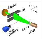
The experimental setup was modified by adding a slit in front of the anode
