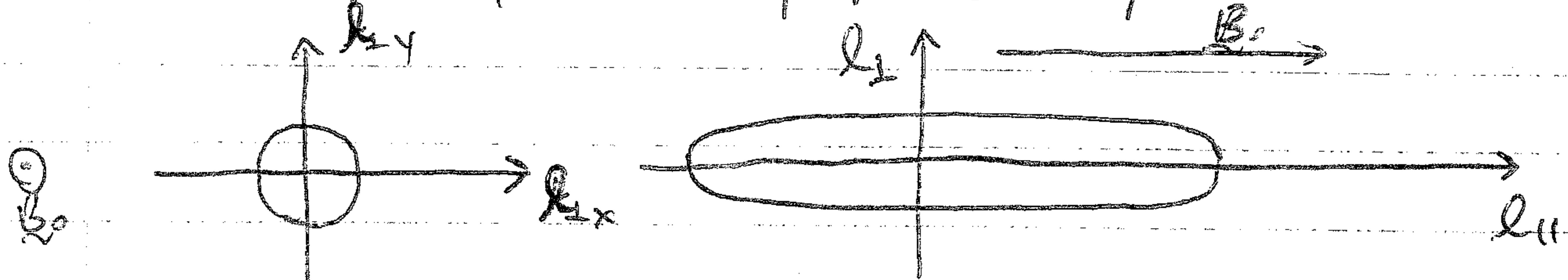
1. Thus, turbulence structures at small scales (with  $k_L \gg k_0$ ) are bimantular, or cigar-shaped, with elongations along the mean magnetic field.
