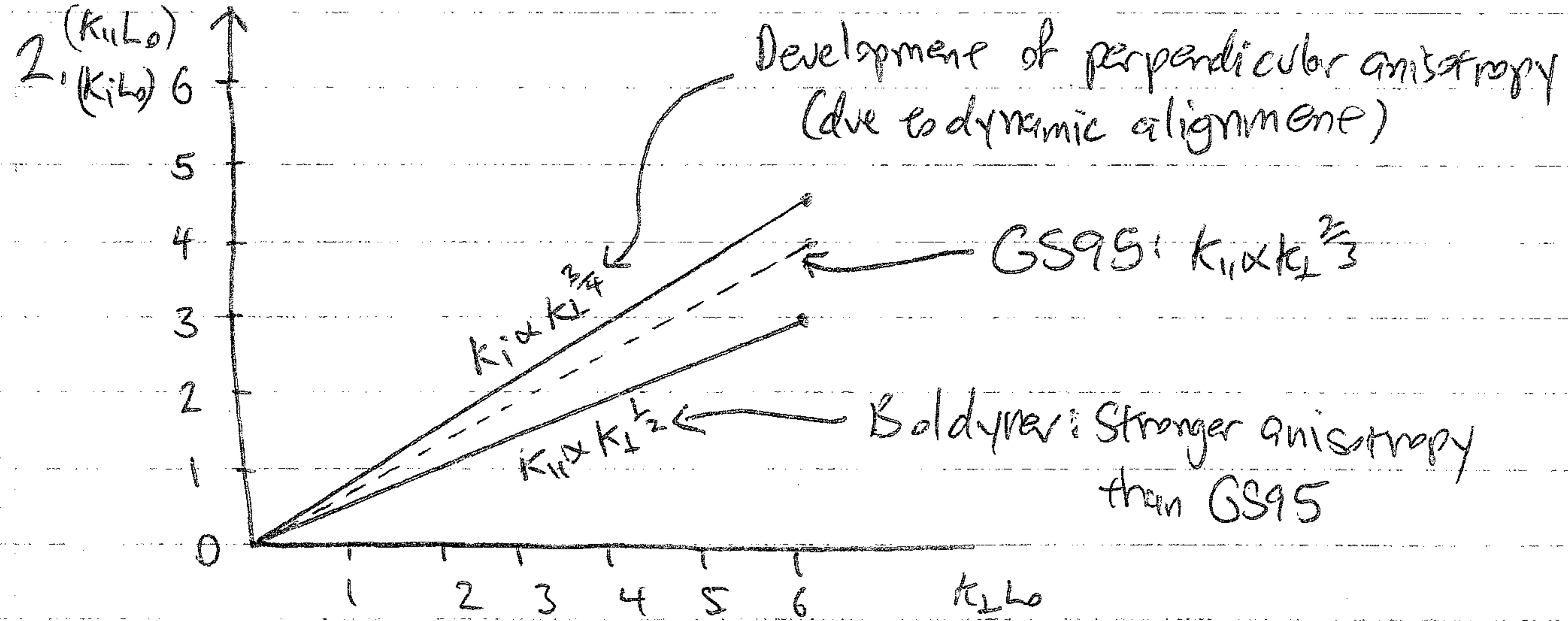
a. Take isotropic driving  $k_{\parallel} = k_x = k_y = k_z = k_0$  with  $V_0 = V_A \Rightarrow \theta_0 = 1$
